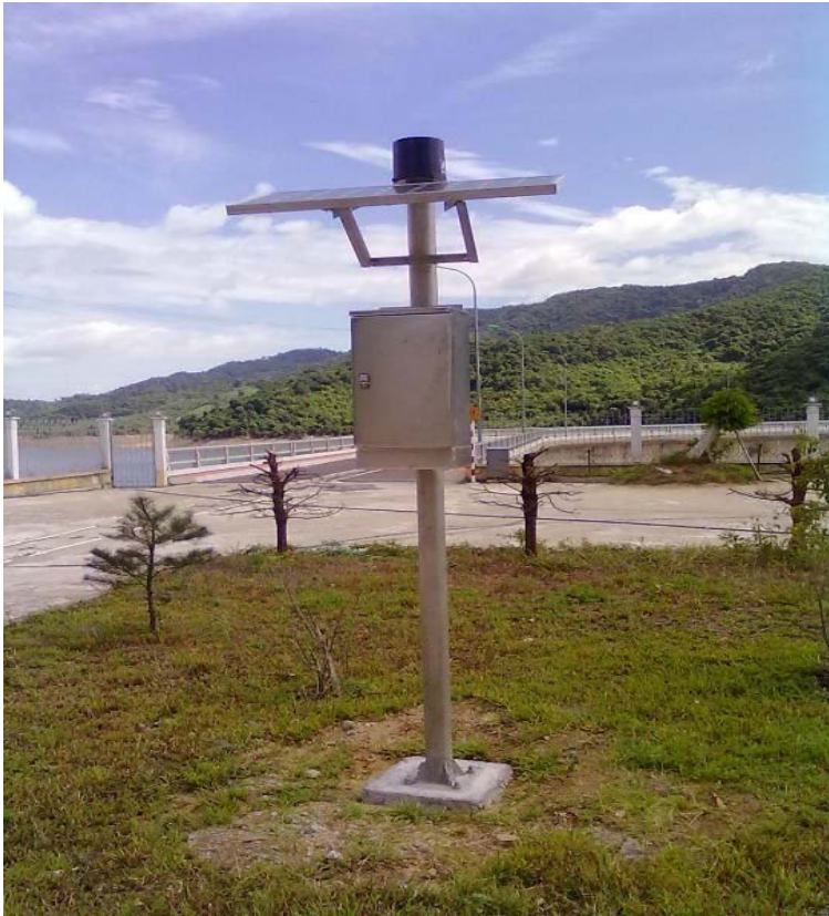
Rain gauge at Dinh Binh reservoir, Southern Central Vietnam
