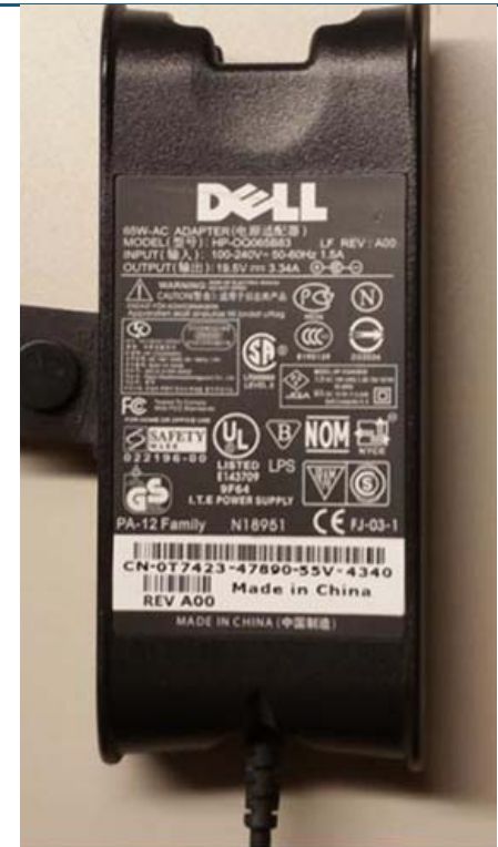
Figure 1. Compliance labeling on a computer power supply may be provided in different ways.
