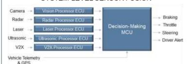
Smart sensors perform data processing and sensorbased decision making locally in the sensor modules. Only processed data is sent back to a central Multipoint Control Unit (MCU) for actionable decision making.
