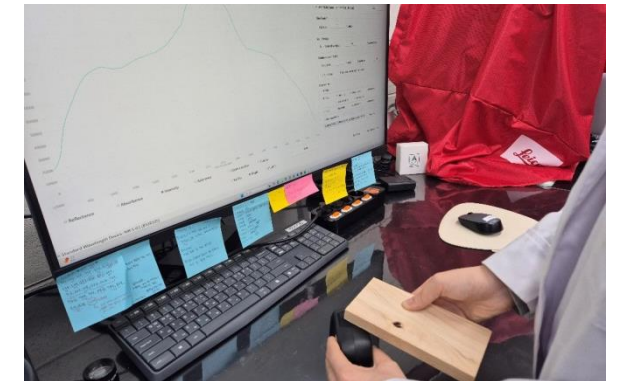
Wood Identification by Portable NIR
